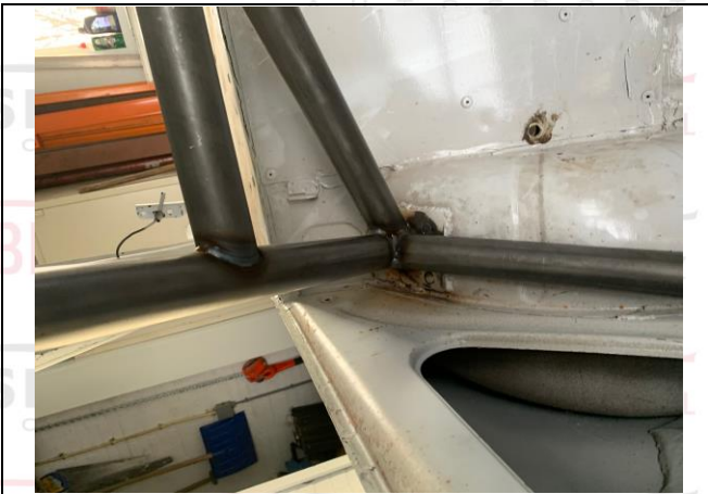
PHOTO 5 REAR BACKSTAY TO BODYSHELL ATTACHMENT
