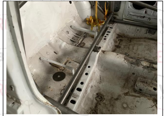
PHOTO 11 ANTI-INTRUSION DOORBAR – CO-DRIVER
