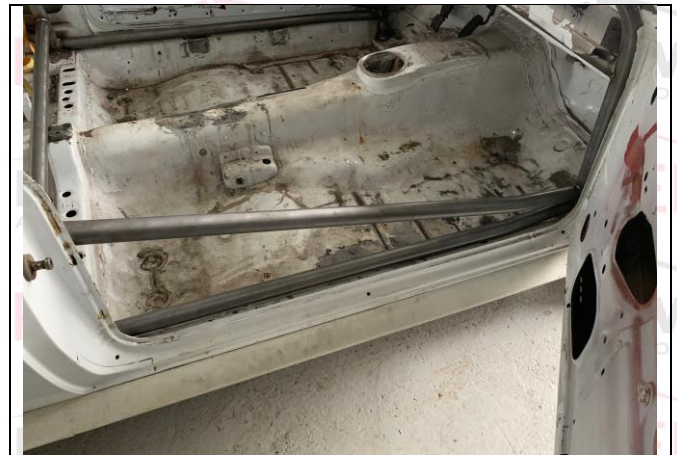
PHOTO 11 ANTI-INTRUSION DOORBAR – CO-DRIVER
