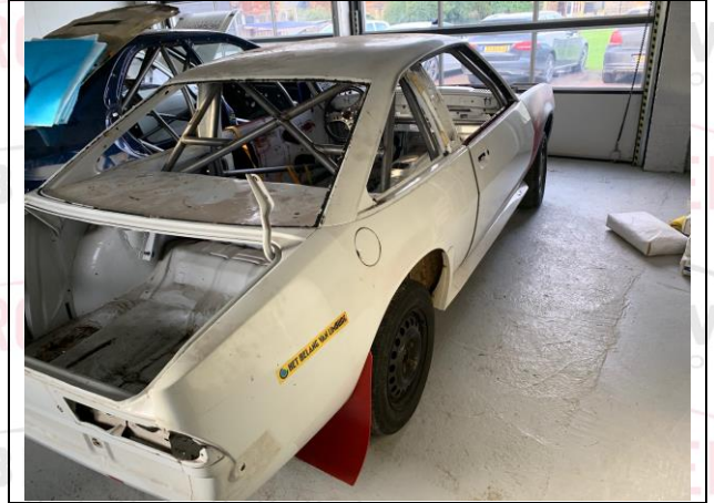
PHOTO 2 REAR ¾ VIEW OF CAGE
