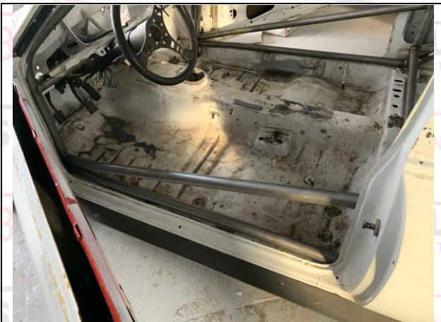
PHOTO 10 ANTI-INTRUSION DOORBAR – DRIVER
