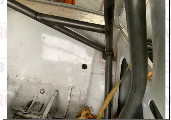
PHOTO 13 SHOULDER HARNESS ATTACHMENT-CO-DRIVER
