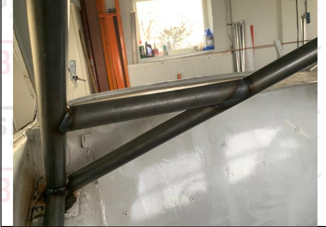
PHOTO 12 SHOULDER HARNESS ATTACHMENT -DRIVER
