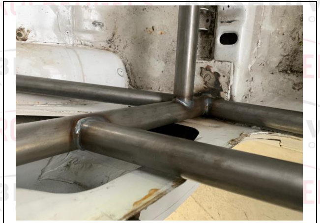
PHOTO 4 MAIN ROLLBAR TO FLOOR ATTACHMENT
