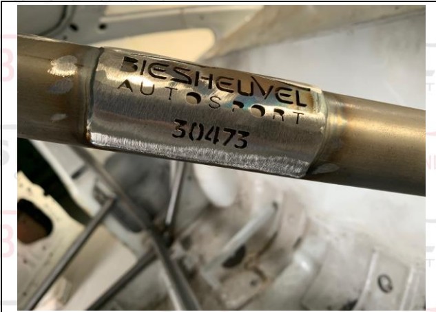
PHOTO 14 DETAIL OF IDENTIFICATION PLATE
